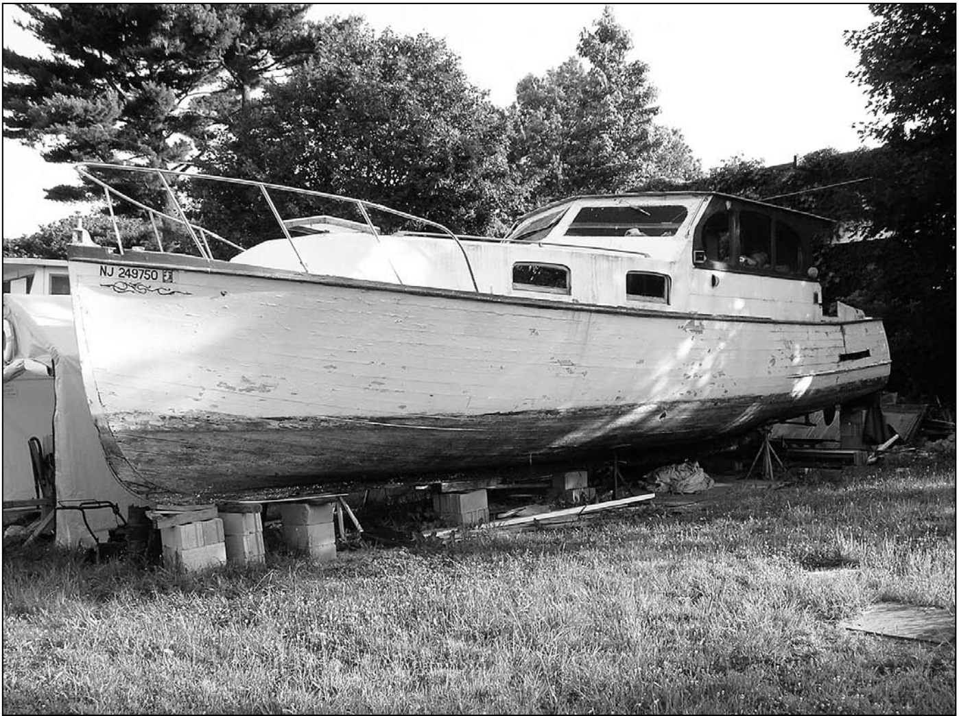
This 39' Consolidated was afloat two years before the photo was taken (summer 2008). The listing stated her twin engines were operable, but the boat was in need of new ribs, floors and deck.
